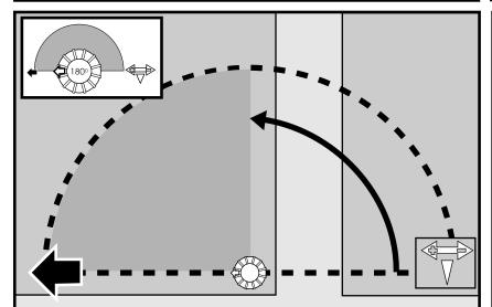
The watering area is between the cap arrow and the right stop arrow on the arc adjustment ring. This example is set to 180°.
